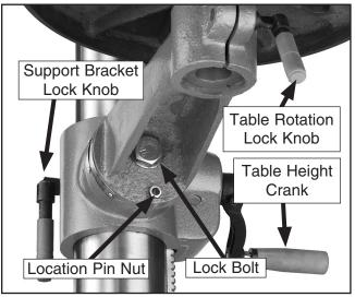
Figure 30. Table adjustment controls.
